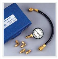
Determine pump efficiency, cut-off and suction, as well as analyze or troubleshoot burner efficiency. Kit includes 2" gauge, 30" 0-150 lb. scale and 12" hose with fittings.
