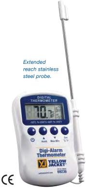
This compact unit measures from -58° to 392°F (-50° to 200°C) and triggers an alarm at the high and low programmed temperatures.
